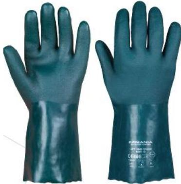
**GLOVE DESCRIPTION:** resistant and flexible PVC gloves, with an additional layer of granular PVC on the hand area to ensure excellent grip in wet and dry environments. The thickness of the glove offers increased resistance to wear and abrasion. The inside of the glove is lined with interlock cotton. The wide cuff facilitates easy removal. The gloves are treated with Actifresh or Sanitized for protection against micro-organisms that cause unpleasant odors or cross-infections. Length 350 mm.
