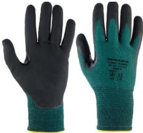
**DESCRIPTION:** machine knitted gloves from a mixture of HPPE fibers and other synthetic fibers, covered with a soft layer of textured nitrile on the palm and fingers, and an additional nitrile start at the base of the thumb; elastic cuff.
